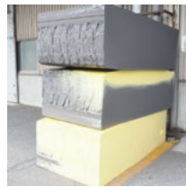
The block in the middle of the urethane foam is the boundary portion generated when changing colors.
