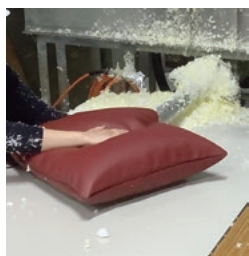
Filling work using chipped urethane (reuse rate: approximately 10.0%)
